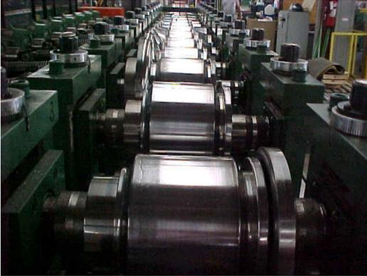
**Roll forming machines** fabricate specific configurations out of long strips of metal, most commonly coiled steel. In most applications, the required cross-section profile of the piece is specifically designed for the machine to bend the metal as necessary. Other than roll forming, these machines perform a number of metalworking duties, including material cutting and roll punching.
