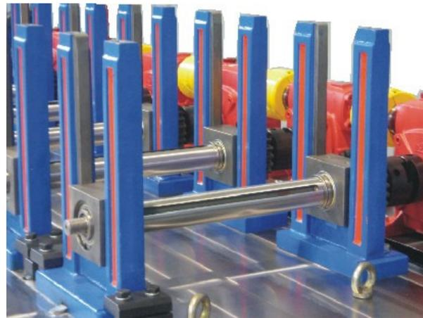
In many modern roll forming machines, programmable logic controllers ensure accuracy. This is vital if a part needs multiple holes or needs to be cut to a specific length. The programmable logic controllers tighten tolerance levels and minimize accuracy.
